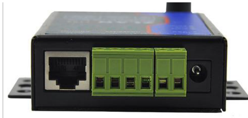
Figure 4 Front Interfaces of ITT-SR-1RS1FE-WiFi
