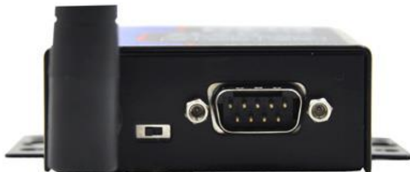
Figure 5 The back of ITT-SR-1RS1FE-WiFi
