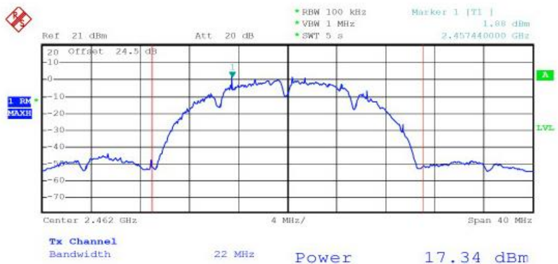
Figure 12 ITT-SR-1RS1FE-WiFi Power Test Curve
